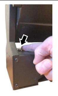
Figure 5. Alignment pin release button
