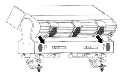
Figure 4. Safety cable attachment points
