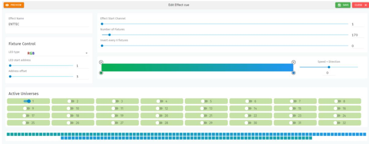
3. Next, define the LED type you want your effect to reference inside the **Fixture Control Tab**, define the LED start address of the first fixture you want the fixture to start on (i.e. the DMX Start address of your first fixture). The Address offset will be populated based on this, however, you can increase this value to leave a larger spacing between each fixture.
