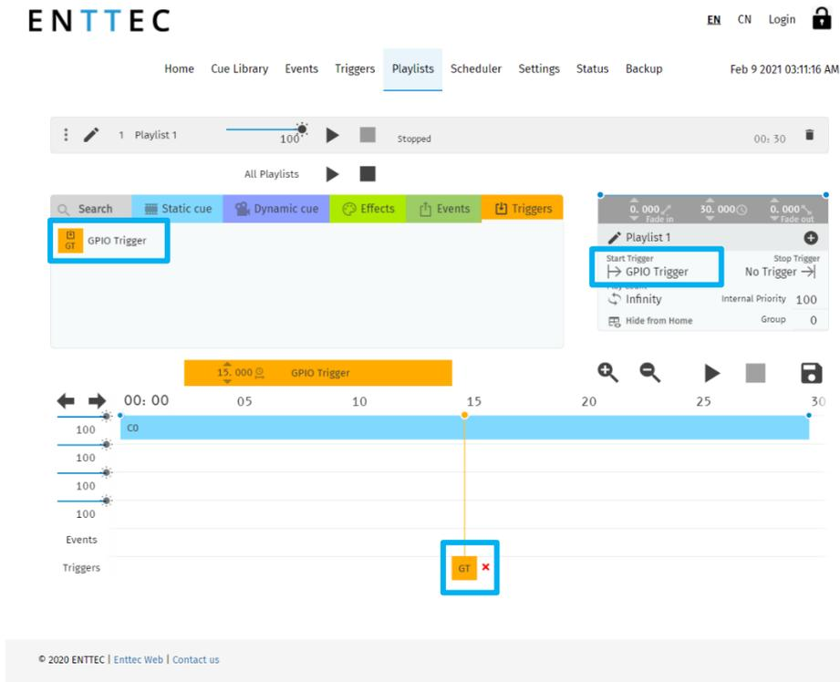
5. The Trigger can be selected as a 'Start Trigger' to commence playback of a certain playlist and/or dragged onto the timeline to act as a condition that must be met for playback to continue.
