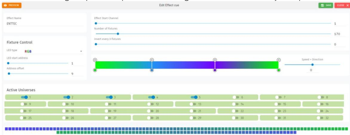
7. Use the toggle switches below the gradient to define the universes that the effect will occupy. This is useful when layering effects or overlapping with other groups. Any universes with switches enabled that the effect does not cover will be saved containing **0** values on each channel when save is pressed.
