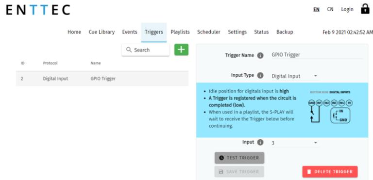
1. Connect a dry input from sensor to Port3 (or any other port), in the GPIO trigger connector in S-PLAY.
