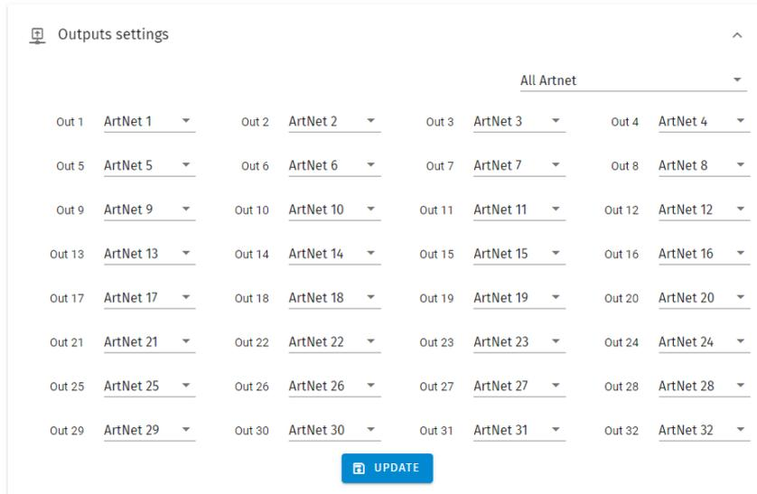
The Output Settings widget allows you to direct data from the S-Play’s 32 internal playback universes to the ArtNet, sACN and DMX configuration tabs lower on the page to create the outputs required for your project.
